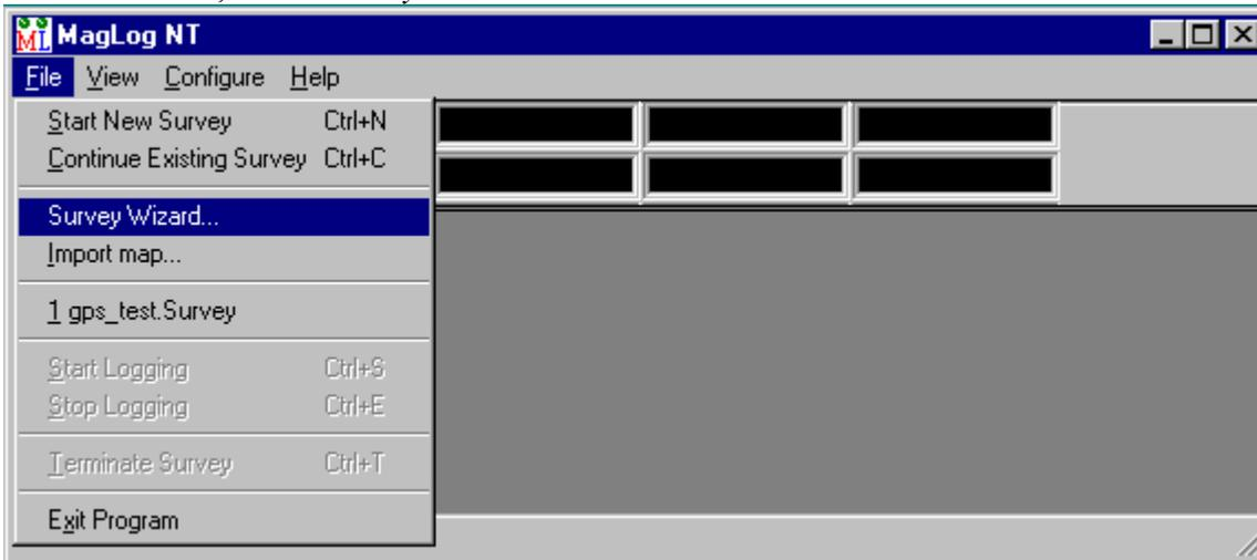
It is recommended that you have your hardware (magnetometer and GPS) connected to the computer and running at this time. GPS should be outputting real positions, and magnetometer also should be running although it may not be producing real measurements at this time (it can be on the ship's deck). If these requirements are not met you still can proceed with *Wizard*, but there is some chance that you may encounter problems in future and have to rerun the wizard when you are under actual survey.
