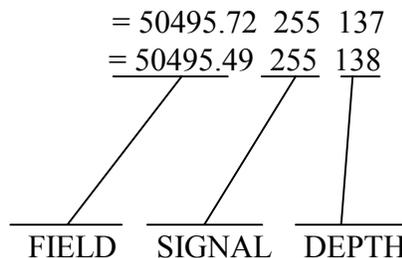
The values shown are for example only and will vary with system configuration. The first reading is the magnetometer field and its value will vary greatly if the sensor is positioned close to a
