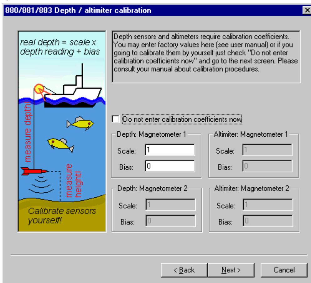
If your hardware includes depth or altimeter sensors, they need to be calibrated. The Wizard does not provide full calibration capabilities (see below how to do depth / altimeter calibration) however it allows entering of the calibration coefficients if you know them. These values might be obtained from the factory or the results of previous calibration procedures. You also can check
