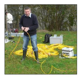
Stewart at the Thur River hydrogeophysical test site in Switzerland in 2010, preparing to deploy a multi-electrode cable for an 18 borehole 3D time-lapse electrical resistivity tomography experiment. The experiment was designed to map electrical resistivity fluctuations induced by infiltrating fresh river water into a saline gravel aquifer. The experiment ran for over one year and yielded travel times and groundwater flow patterns.
