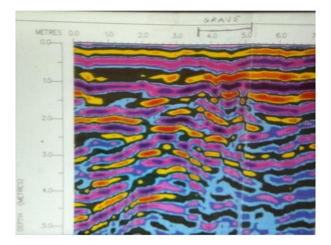
Figure 3Showing some of the typical shallow GPR features found in Tentland - such as<br/>tree roots, pipes and other infrastructure, possible burials
